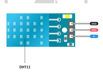
**VCC:** Pin provides power to the sensor. Despite the fact that the supply voltage of the module ranges from 3.3V to 5.5V, a 5V supply is recommended. With a 5V power supply, the sensor can be placed up to 20 meters away. With 3.3V supply voltage, the sensor can be placed just 1 meter away; otherwise, the line voltage drop will cause measurement errors.
